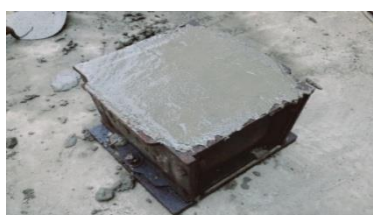
Fig. 1 Copper slag concrete cube of size 150 mm × 150 mm × 150 mm
